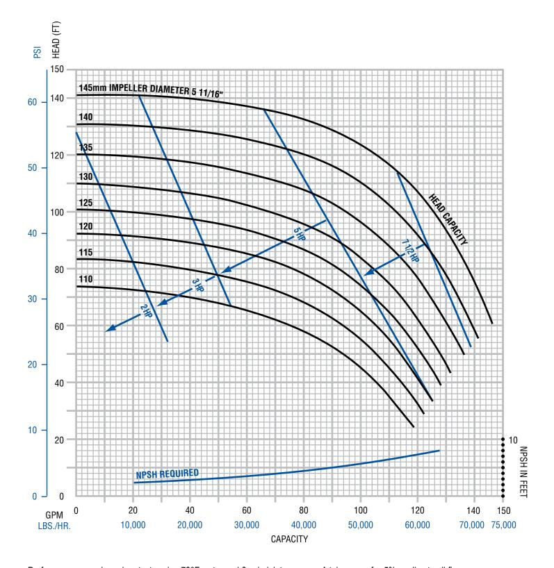
Performance curve based on tests using 70°F water and 0 psig inlet pressure. A tolerance of ± 5% applies to all figures. Actual performance may vary by application product. Please contact Fristam for different conditions.
